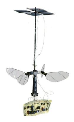
Changes to the Robobee -- including an additional pair of wings and improvements to the actuators and transmission ratio -- made the vehicle more efficient and allowed the addition of solar cells and an electronics panel. This Robobee is the first to fly without a power cord and is the lightest, untethered vehicle to achieve sustained flight. Credit: Harvard Microrobotics Lab/Harvard SEAS
