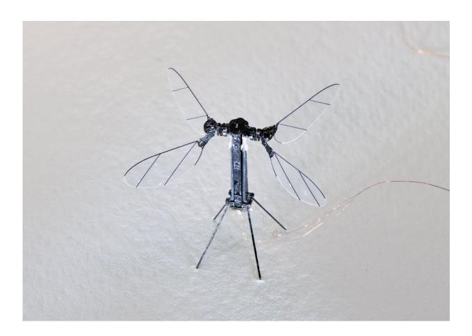
The RoboBee X-wing has four wings driven by two piezoelectric actuators. The vehicle has a total wingspan of 3.4 cm, weighs 90 mg, and has a maximum lift of 370mg. Credit: Noah T. Jafferis and E. Farrell Helbling, Harvard Microrobotics Laboratory
