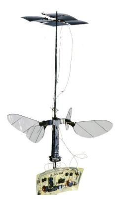
Changes to the Robobee -- including an additional pair of wings and improvements to the actuators and transmission ratio -- made the vehicle more efficient and allowed the addition of solar cells and an electronics panel. This Robobee is the first to fly without a power cord and is the lightest, untethered vehicle to achieve sustained flight. Credit: Harvard Microrobotics Lab/Harvard SEAS
