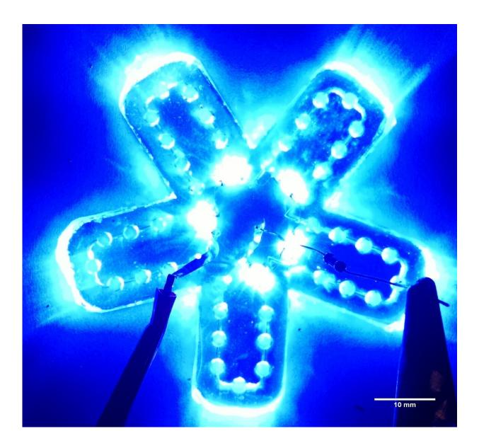
Fluorescent proteins expressed by bacteria on the bacteria-operated robotic gripper. Credit: Justus et al., Sci. Robot. 4, eaax0765 (2019)
