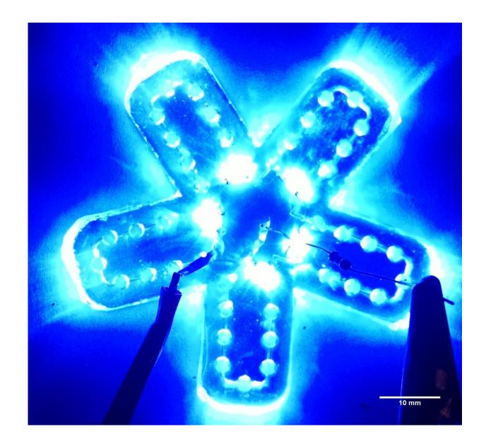
Fluorescent proteins expressed by bacteria on the bacteria-operated robotic gripper. Credit: Justus et al., Sci. Robot. 4, eaax0765 (2019)
