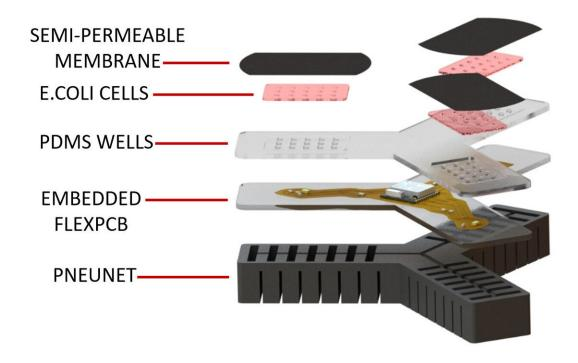
Deconstructed view of the bacteria-operated robotic gripper. Credit: Tess Hellebrekers
