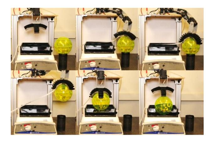
This robotic gripping arm uses engineered bacteria in wells in its fingers to 'taste' for a specific chemical before deciding whether to pick up the ball and put it in the bath. The system was developed by engineers at UC Davis and Carnegie Mellon University. Credit: Tess Hellebrekers, Soft Machines Lab, Carnegie Mellon University
