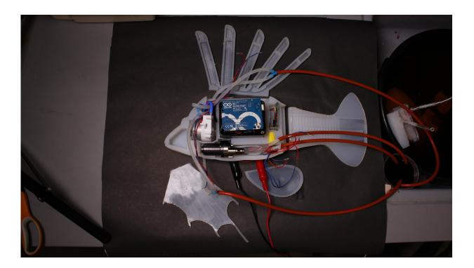
Electronic innards of soft robotic fish, showing pumps, molded silicone shell with fin actuators, microcontrollers, and catholyte vasculature. Credit: James Pikul
