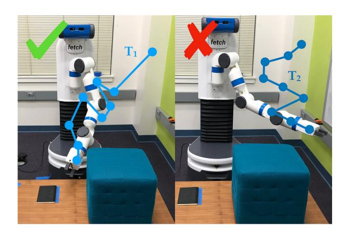
An example of how the robot arm uses survey questions to determine the preferences of the person using it. In this case, the person prefers trajectory #1 (T1) over trajectory #2. Credit: Andy Palan and Gleb Shevchuk
