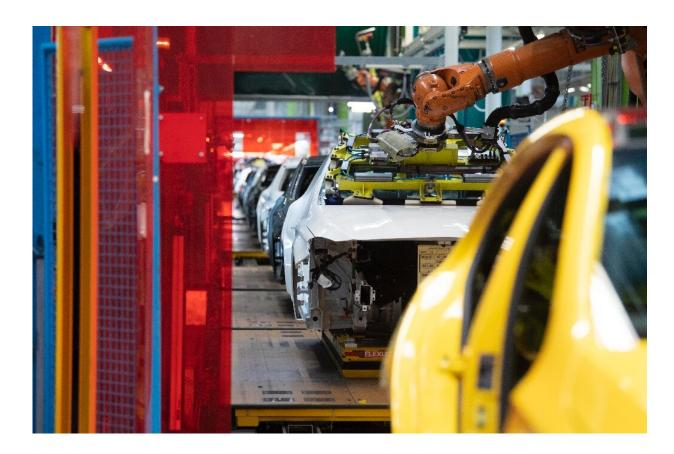
A robot mounts a windshield on a Mercedes Benz A Class on the assembly line at the Daimler AG factory in Rastatt, southwestern Germany, an example of the numerous tasks that are being automated as a result of new technologies
