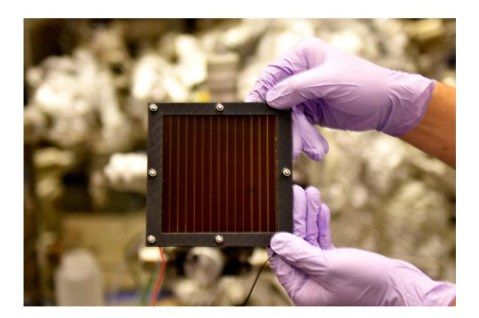
This perovskite solar module is better able to contain the lead within its structure when a layer of epoxy resin is added to its surface. This approach to tackling a long-standing environmental concern helps bring the technology closer to commercialization. Credit: OIST
