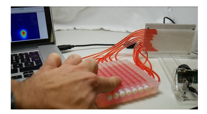
The touchpad developed using Skinflow. Credit: Soter et al.
