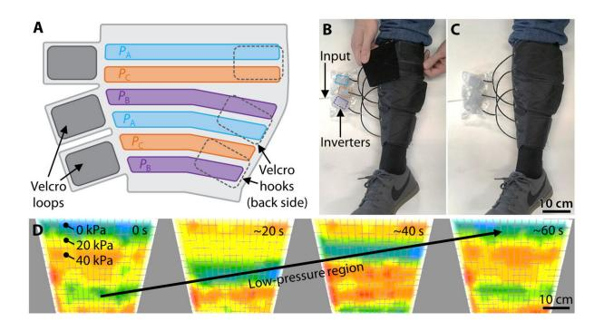
Use of the soft ring oscillator to control an inflating mechanotherapeutic device applied to the lower leg. Credit: Preston et al., Sci. Robot. 4, eaaw5496 (2019)
