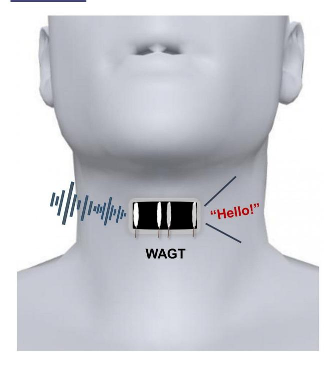
A wearable artificial graphene throat, abbreviated here as 'WAGT,' can transform human throat movements into different sounds with training of the wearer. Credit: Adapted from *ACS Nano* **2019**, 10.1021/acsnano.9b03218
