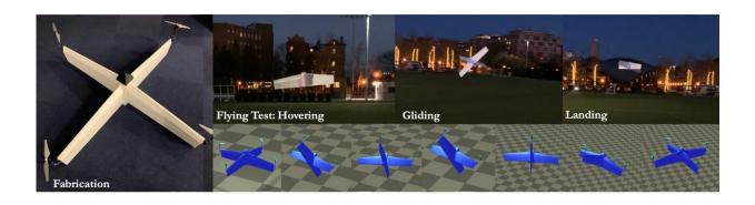
Hybrid unmanned aerial vehicles, or UAVs, are drones that combine the advantages of multi-copters and fixed-wing planes. These drones are equipped to vertically take off and land like multi-copters, yet also have the strong aerodynamic performance and energy-saving capabilities of traditional planes. As hybrid UAVs continue to evolve, however, controlling them remotely still remains a challenge. Credit: Jie Xu
