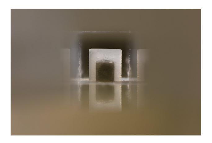
The cupula (light area) within the acrylic channel used for experimental testing. Inside the cupula are liquid metal gallium-indium plates (dark area). Credit: U.S. Naval Research Laboratory.
