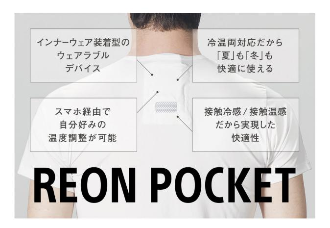
Sony has come up with a wearable air conditioner. It's called the Reon Pocket. It is a tiny AC unit that fits right inside the shirt. The device takes a battery; the person adjusts the temperature by smartphone via a
