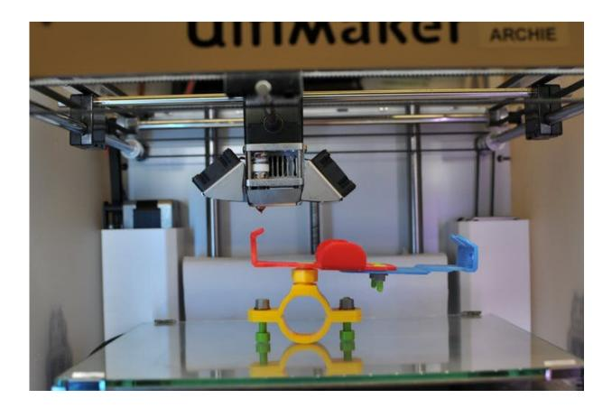
A custom designed phone holder for a bicycle, assembled from 3-D printed components. Credit: 4Delta, Author provided
