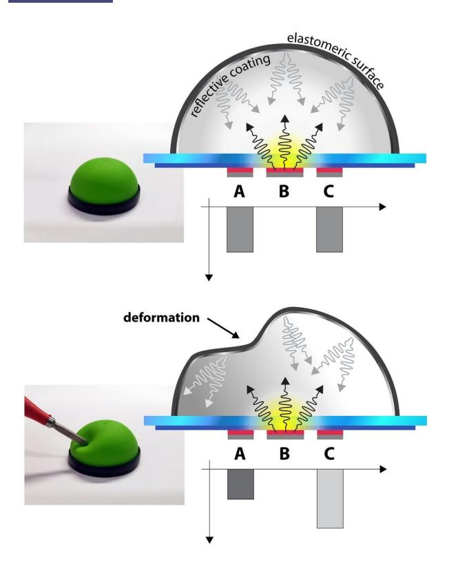
A single touch element made up of a dome over some OLED pixels. Top, when
