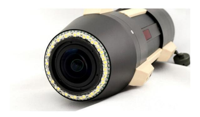
The wireless device is placed into a tube, and the image from the camera is sent to a computer screen Credit: D-TEST
