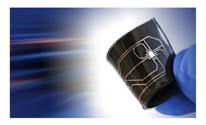
Researchers at the Soft Machines Lab have developed a soft magnetic skin with a single sensing element that detects force and contact. Credit: College of Engineering, Carnegie Mellon University
