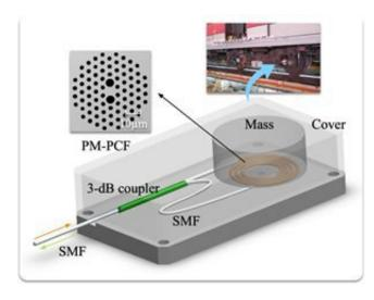
The new fiber-optic accelerometer features a polarization-maintaining photonic crystal fiber that is coiled into the shape of a disc only 15 millimeters in diameter. When a vibration occurs, the mass block presses on the coiled fiber at a frequency matching that of the vibration. This external force causes the wavelength of light in the fiber to shift in a measurable way. Credit: The Hong Kong Polytechnic University
