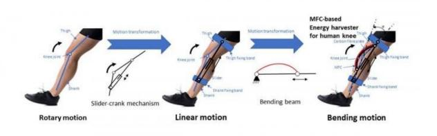
Diagram of the slider-crank mechanism that generates energy during the knee's motion. Credit: Gao et al.
