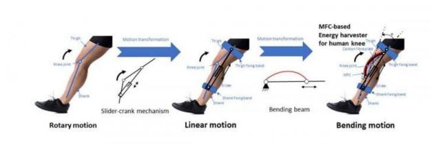
Diagram of the slider-crank mechanism that generates energy during the knee's motion. Credit: Gao et al.
