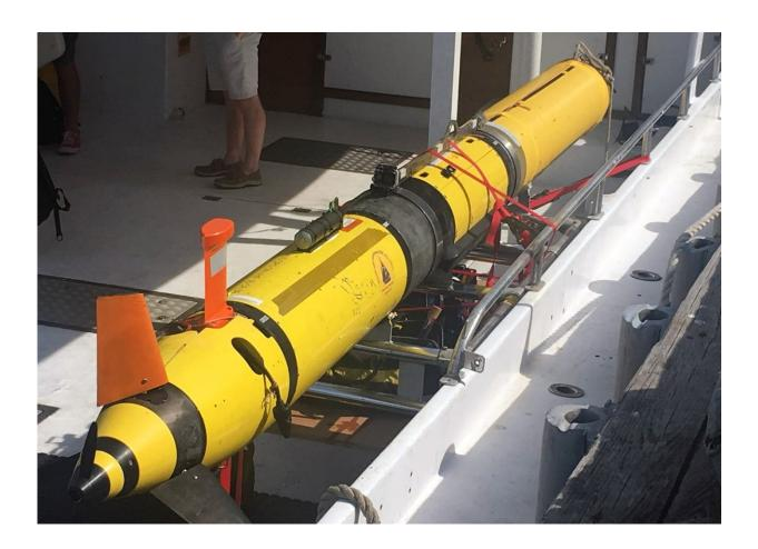
WHOI researchers deployed a REMUS 600 AUV to survey a subsea cable system in Buzzards Bay, Mass. The vehicle uses a propeller and fins for steering and diving, and relies on an internal navigation system to independently survey swaths of the ocean. Credit: Evan Lubofsky, Woods Hole Oceanographic Institution
