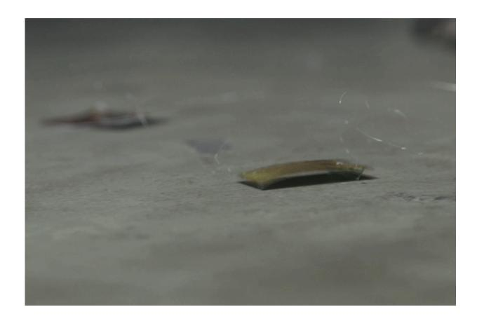
The robot is built of a layered material that bends and straightens when AC voltage is applied, causing it to spring forward in a "leapfrogging" motion. Credit: UC Berkeley photo by Stephen McNally
