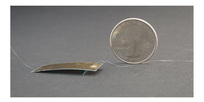
A new insect-sized robot created by researchers at the University of California, Berkeley, scurries at the speed of a cockroach and can withstand the weight of a human. Credit: UC Berkeley photo by Stephen McNally
