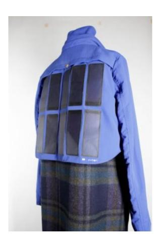
Pvilion's flexible solar panels can be integrated into clothing, as shown with this prototype jacket. Credit: Syracuse University
