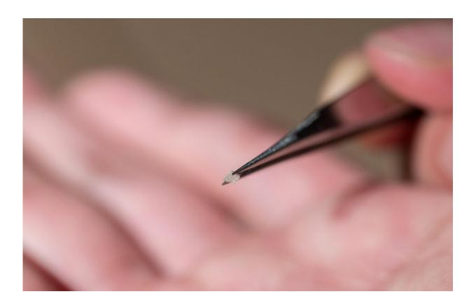
Close-up photo shows a micro-bristle-bot, which is about two millimeters in length – about the size of the world's smallest ant. Credit: Allison Carter, Georgia Tech
