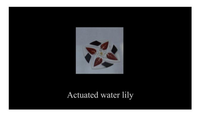
The printed water lily is placed at fluid interfaces and actuated using a permanent magnet. Credit: Science Advances, doi: 10.1126/sciadv.aaw1160
