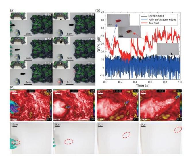
(a) Photographs of a robot targeting an LED-indicated path. The targeting demonstration shows the accuracy that the robot control can achieve. (b) Comparison of the measured relative noise level of a soft macro robot and a battery-powered, similarly sized toy boat. RSPL denotes to the relative sound pressure level. The robot exhibits a much lower noise level compared to the toy
