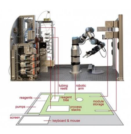
Guided by artificial intelligence and powered by a robotic platform, a system developed by MIT researchers moves a step closer to automating the production of small molecules. Credit: Connor Coley, Felice Frankel
