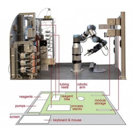
The new system combines three main steps. First, software guided by artificial intelligence suggests a route for synthesizing a molecule, then expert chemists review this route and refine it into a chemical "recipe," and finally the recipe is sent to a robotic platform that automatically assembles the hardware and performs the reactions that build the molecule. Credit: Connor Coley, Felice Frankel
