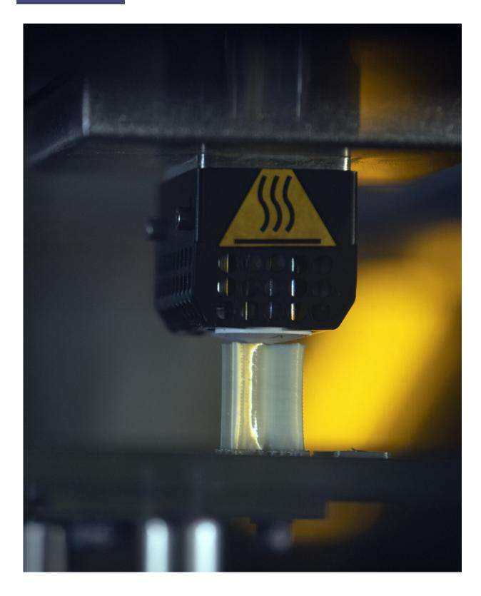
An aircraft part prints on the Stratasys F900 three-dimensional printer Aug. 15, 2019, at Travis Air Force Base, California. Travis AFB is the first field-unit
