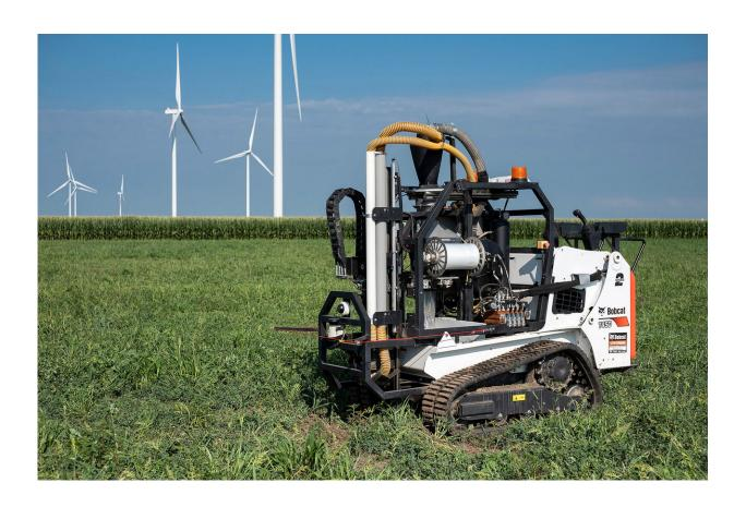
A pair of Purdue University graduates have founded a company called Rogo Ag LLC, a pioneering agricultural technology company that has developed an autonomous robot called Smartcore. Smartcore is designed to collect accurate, repeatable soil samples in fields and bring the samples directly to the farmers or growers. Credit: Purdue Research Foundation image/Oren Darling
