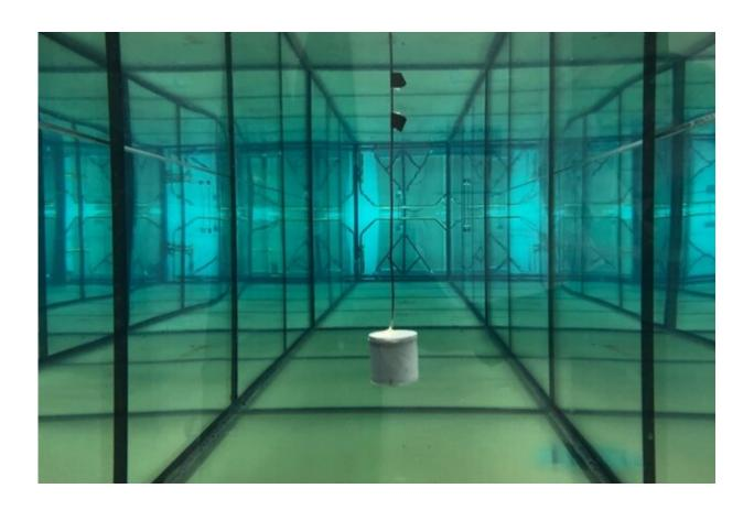
A battery-free underwater "piezoelectric" sensor invented by MIT researchers transmits data by absorbing or reflecting sound waves back to a receiver, where a reflected wave decodes a 1 bit and an absorbed wave decodes a 0 bit — and simultaneously stores energy. Credit: Massachusetts Institute of Technology
