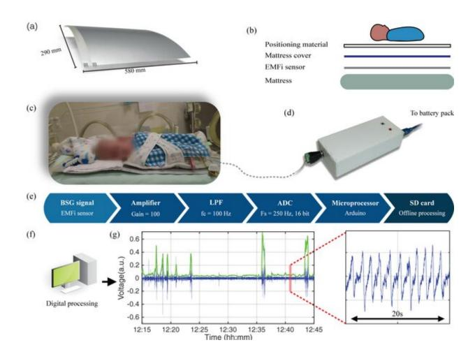
The film-like pressure sensor (a) is embedded in the mattress (b) of the incubator (c) and connected to the signal acquisition system (e), which is powered by a battery pack (d). The acquired signal is processed by a computer (f) which displays the infant-motion (g, green) and the breathing rate (g, blue). Credit: Joshi et al., 2018
