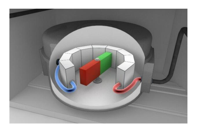
© Fraunhofer IPM Setup of a magnetocaloric cooling system: The segments shown in gray contain the magnetocaloric material. This material is alternately heated and cooled by the rotating magnet. Because of the internal structure of the segments, heat is transferred to the ambient air on the right side while on the left heat is removed from the container to be cooled.
