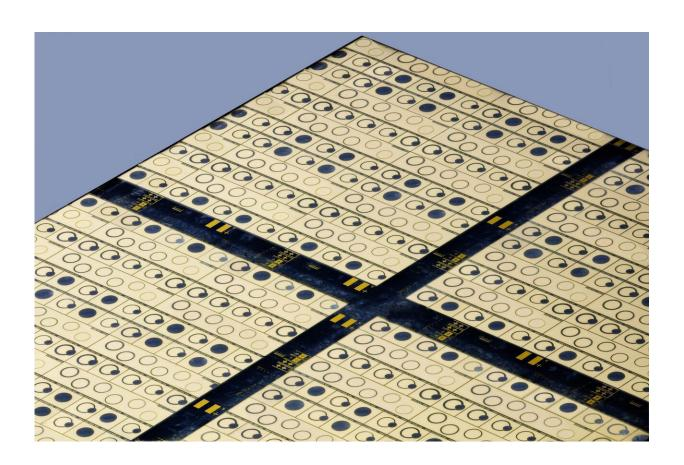
Gallium oxide chip with transistor structures and for measurement purposes, processed at FBH via projection lithography. Credit: FBH/schurian.com
