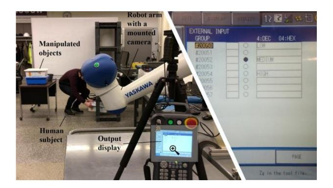
To test how well the algorithm might work in a warehouse, the researchers had a robot (white arm) monitor 10 participants performing activities in a warehouse-like setting. Within three seconds of the end of each activity, the robot showed a score on its display (right). Credit: Parsa et al./IEEE Robotics and Automation Letters
