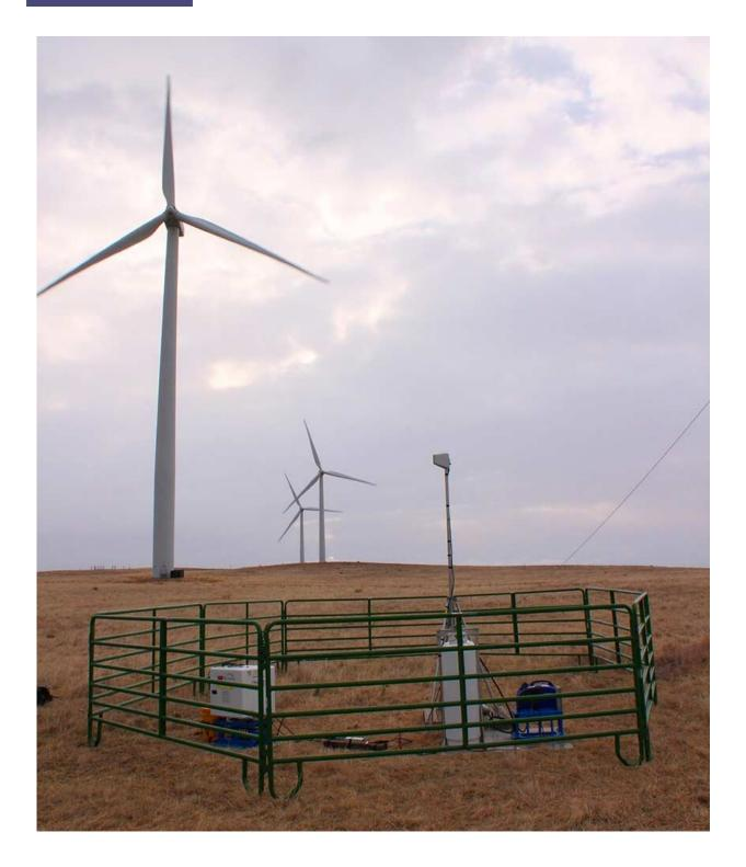
NREL's experimental design for the wake steering field campaign incorporated lidar measurements of atmospheric conditions. Credit: Andrew Scholbrock, NREL
