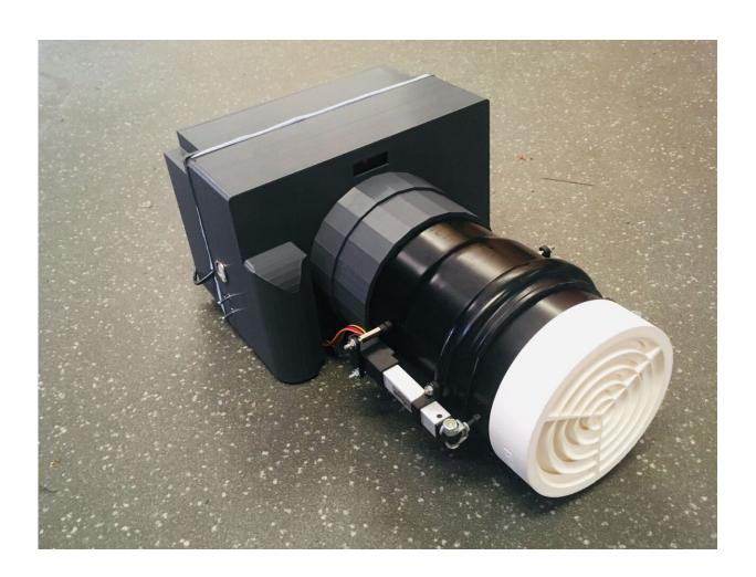
The current version of Sussex's acoustic projector. The speaker is contained in the back, together with the tracking camera and one of the acoustic lenses. The part in white is the second acoustic lens in the telescope. Credit: University of Sussex
