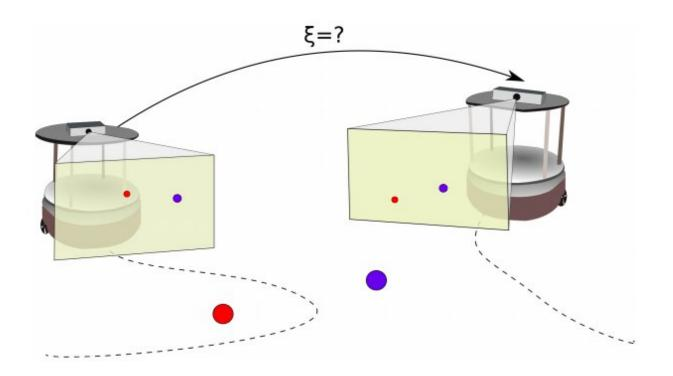
A representation of the problem addressed in the recent study. Two robots are observing a pair of 3D points. The researchers propose a pipeline to simultaneously estimate the 3D depth of the two 3D points and simultaneously obtain their relative pose. Credit: Rodrigues et al.
