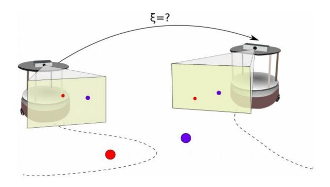
A representation of the problem addressed in the recent study. Two robots are observing a pair of 3D points. The researchers propose a pipeline to simultaneously estimate the 3D depth of the two 3D points and simultaneously obtain their relative pose. Credit: Rodrigues et al.
