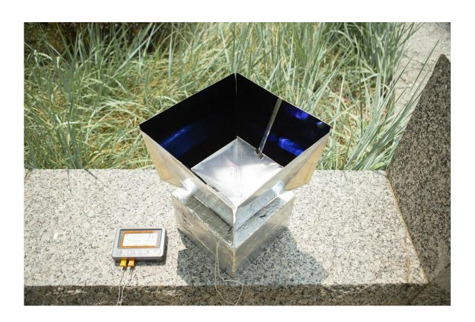
The system helps cool its surroundings by absorbing heat from the air inside the box and transmitting that energy through the Earth's atmosphere into outer space. Credit: University at Buffalo
