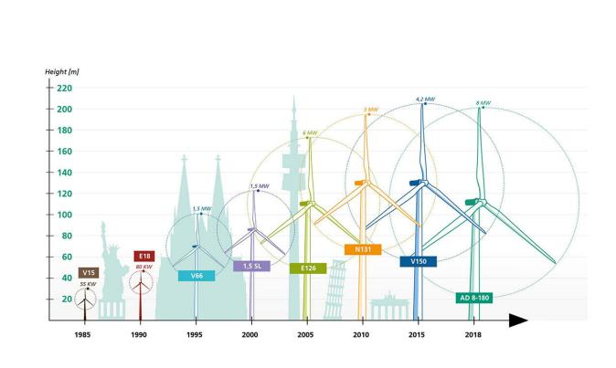
The growth in wind energy solutions, with larger, more efficient wind turbines over the decades. Credit: Fraunhofer IWES
