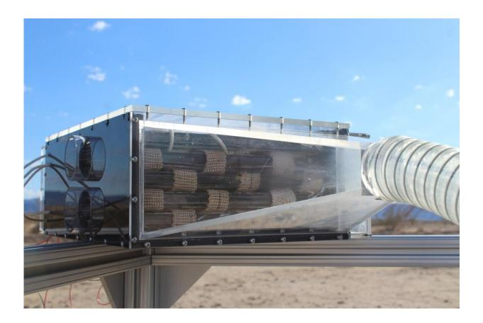
The latest version of UC Berkeley's water harvester blows ambient air over a cartridge filled with MOF, which is visible inside the plexiglass box. The MOF pulls water from arid air, which is then removed from the MOF by mild heating. The concentrated water vapor is blown out through the tube at right to a condenser. This process produces water for drinking using only solar panels and a battery, even in areas as dry as the Mojave Desert. Credit: Mathieu Prévot, UC Berkeley
