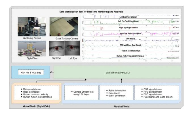
A system diagram of the implementation based on the proposed framework representing the data collection and monitoring during an HRC experiment. Credit: Savur, Kumar & Sahin.
