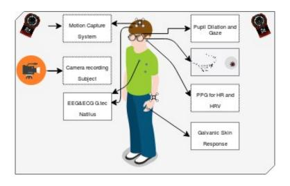
Sensors and devices used in the prototype implementation. The researchers used a motion capture system to monitor human motion and a camera to record the experiment. They also tracked human-gaze using Pupil Labs and human physiological responses such as pupil dilation, PPG, GSR, EEG \& ECG recorded. Credit: Savur, Kumar & Sahin.
