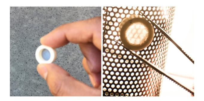
Laser welded ceramic assembly consisting of a transparent cylindrical cap joined to a ceramic tube. Credit: Garay lab/UC San Diego Jacobs School of Engineering
