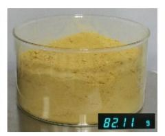
Synthesis at small scale (82.11 grams of product). Note that the reaction is carried out in a beaker open to air. Credit: Vepa Rozyyev/Texas A&M University
