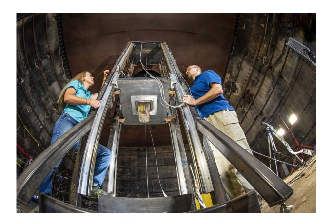
Sandia National Laboratories engineers June Stanley and Chris Grosso demonstrate how the drop tower they built abuses batteries to understand how the lithium-ion cells respond to different types of stress. Credit: Randy Montoya
