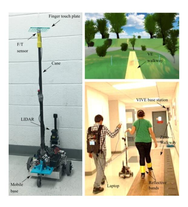
(Left) A view of CANINE. The LIDAR was positioned at the rear of the robot
