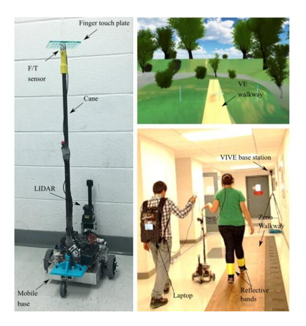
(Left) A view of CANINE. The LIDAR was positioned at the rear of the robot
