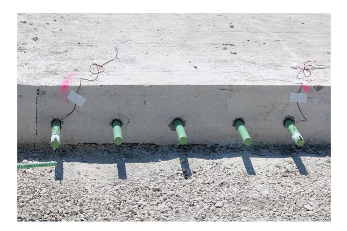
Sensors developed by Purdue engineers are being embedded into Indiana highways to determine when concrete is mature enough to open up traffic following a construction project. Credit: Purdue University photo/Erin Easterling
