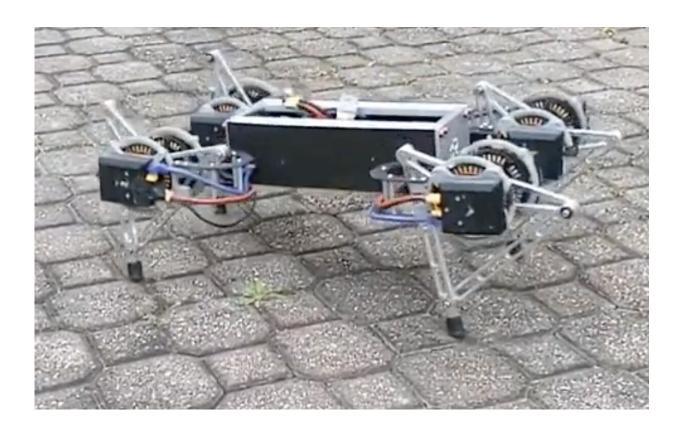
The robot used in this experiment was a Minitaur brand machine with legs. Credit: Georgia Tech / Neveln
