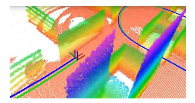
The team built a 3-D plane-based map using a 3-D LiDAR and an inertial sensor. LiDAR is like radar but uses light instead of radio waves. Points with different colors are the different planes (which serve as the landmarks for navigation), the green line is the true trajectory and the blue line is the estimated trajectory computed by the team's simultaneous localization and mapping (SLAM) algorithm. Credit: University of Delaware
