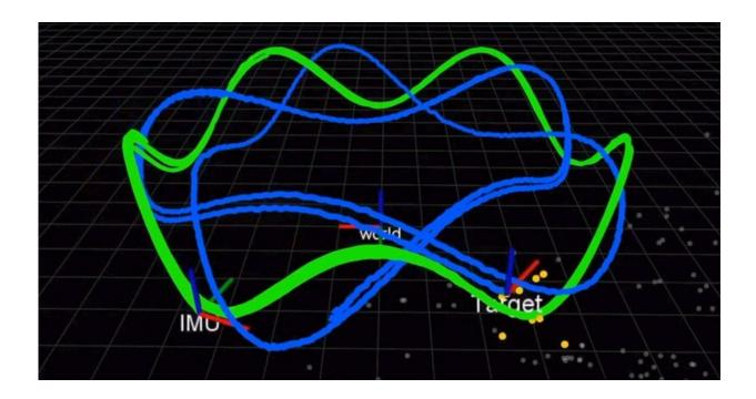
The team uses a camera and an inertial measurement unit (IMU) to simultaneously localize a robot and track a moving target. The green line is the robot's trajectory and the blue line is the target's trajectory. Credit: University of Delaware
