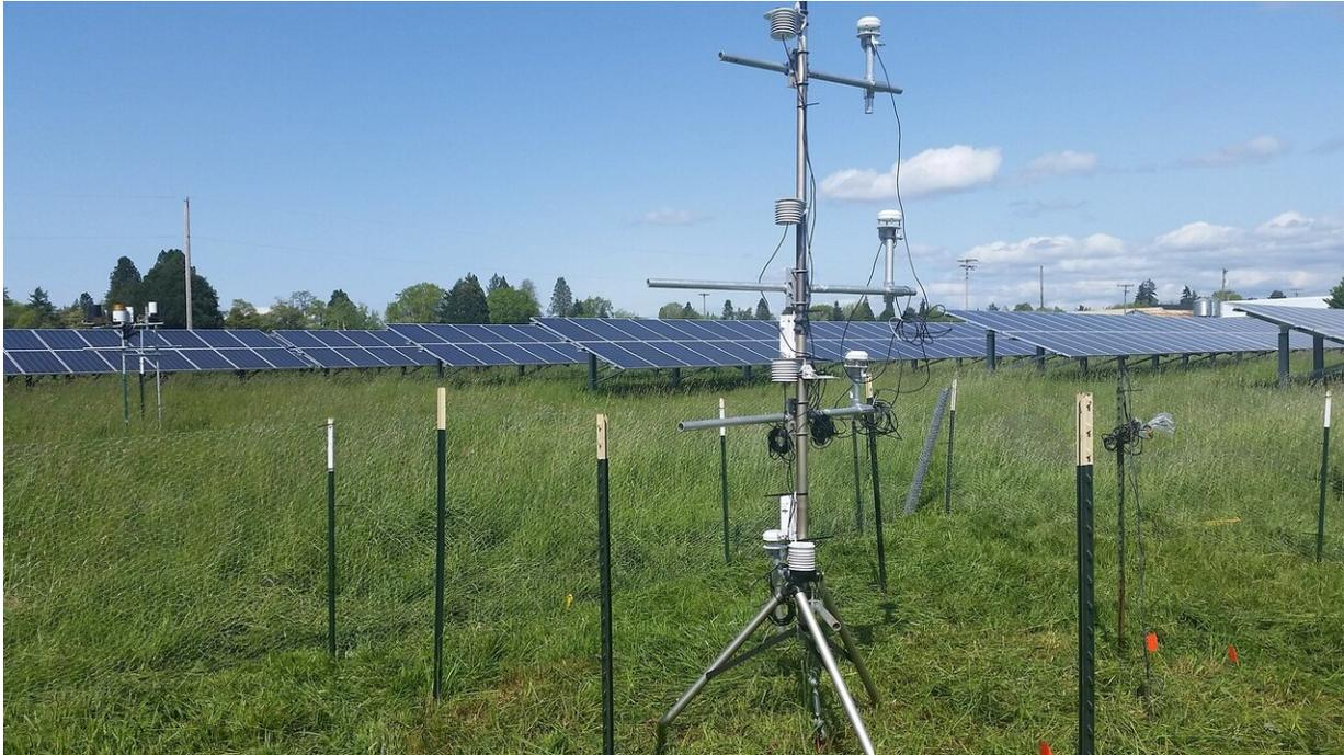
Researchers installed meteorological instruments in and adjacent to the 35th Street Solar Array at Oregon State University to measure temperature, relative humidity, wind speed wind direction and incoming solar energy. Photo by Elnaz Hassanpour. Credit: Elnaz Hassanpour, Oregon State University
