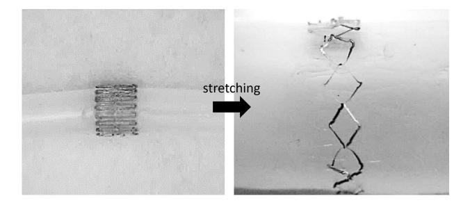
The wireless blood flow sensor is stretchable, allowing it to conform to a stent for implantation. Credit: Georgia Tech
