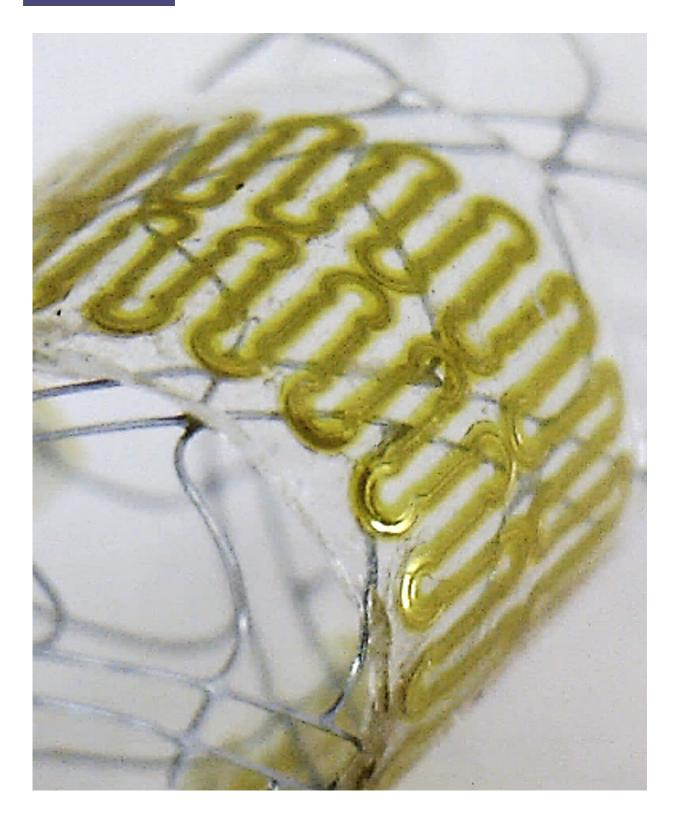
This close-up image shows details of the ultra-thin, low-profile sensor for monitoring blood flow in the brain. Credit: Georgia Tech
