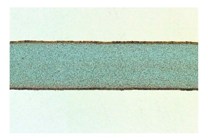
MIT researchers have 3-D printed ultrathin ceramic films that convert energy from one form into another for flexible electronics and biosensors. The process involves printing long, narrow lines of "piezoelectric" feedstock (pictured) on a substrate, overlapping the lines, and drying them out at room temperature. Credit: Massachusetts Institute of Technology
