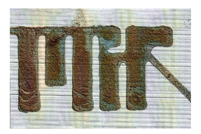
MIT researchers have 3-D printed ultrathin ceramic films that convert energy from one form into another for flexible electronics and biosensors. Here, they've printed the piezoelectric films into a pattern spelling out "MIT." Credit: Massachusetts Institute of Technology
