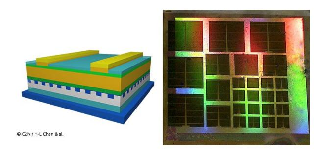
(left) Sketch of an ultrathin solar cell made of GaAs with a nanostructured back mirror. (right) Photograph of a sample showing the diffraction effect of a nanostructured mirror in air (colored shine) and the absorption enhancement effect in ultrathin solar cells (square black areas). Credit: © C2N / H-L Chen & al.
