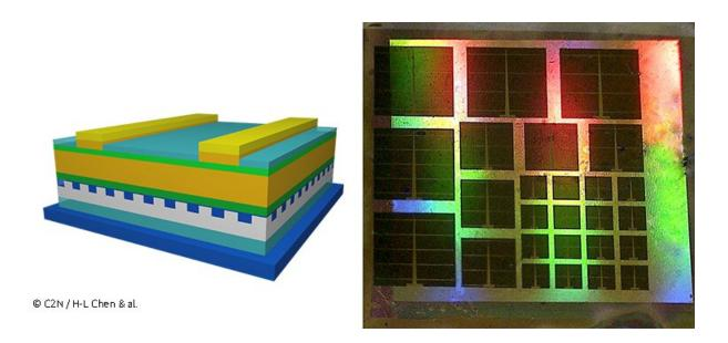
(left) Sketch of an ultrathin solar cell made of GaAs with a nanostructured back mirror. (right) Photograph of a sample showing the diffraction effect of a nanostructured mirror in air (colored shine) and the absorption enhancement effect in ultrathin solar cells (square black areas). Credit:  $\bigcirc$  C2N / H-L Chen & al.
